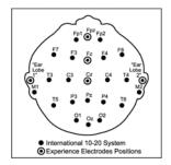
Figure 3. International 10-20 System (Electrodes' Position)
