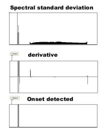
Figure 11. Visualization of spectral standard deviation event detection function, the discrete derivative and the event detection
