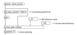
Figure 8. Gated spectral standard deviation, event detection function
