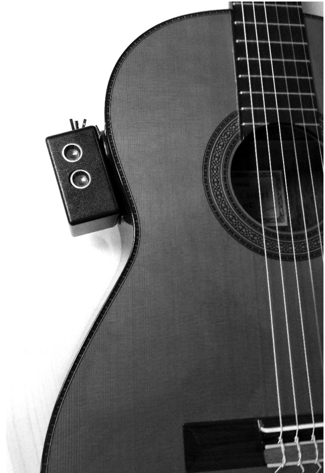
Figure 1: GuitarAMI new prototype, constructed using the ESP8260 WiFi microcontroller, ultrasonic sensor and accelerometer.
